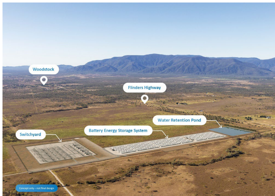
Artist impression of the Supernode North BESS. Please note the Water Retention Pond is proposed to manage stormwater runoff on site.
